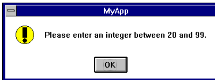
Figure 10 - The error message displayed by the MFC function DDV_MinMaxInt() .
