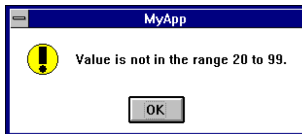
Figure 9 - The error message displayed by an ObjectWindows TRangeValidator object.
